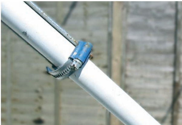
● Fig. 6 (left): Each spreader is simply clamped to the spider with two 'Jubilee' clips as shown in Fig. 2.
