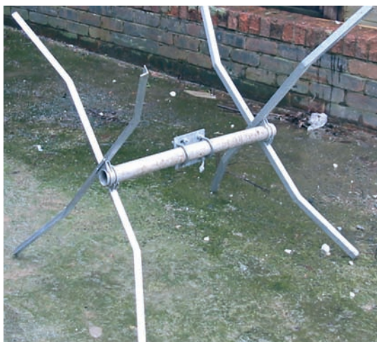
● Fig. 4: The completed spider and boom assembled with only the spreaders needing to be fitted (see text).
