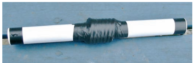
● Fig. 8: After the traps are held in place with tightly wrapped pvc insulating tape, they are ready to have the heavy duty waterproofing Denso tape wrapped around them.
